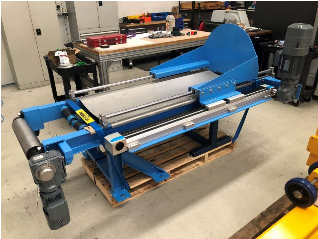
Tank up-ender for manufacturing line
